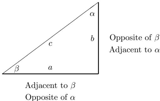
$$\begin{aligned}\sin \beta &= \frac{b}{c} = \cos \alpha \\ \csc \beta &= \frac{c}{b} = \sec \alpha\end{aligned}$$
